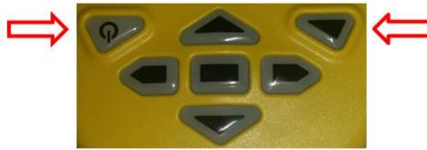
Figure 1: How to Hard Reset your MMS7000 device
